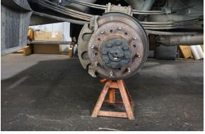
**4.** Use brake cleaner and wire brush to clean any dirt and surface rust off factory studs and mounting surfaces.
