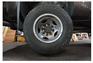
**3.** Remove the rear wheels with a 22mm socket and impact wrench.
