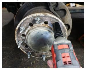
**6.** Cut the studs at the paint marker line. <u>The studs will be hot! Use caution before touching</u> them and wait until they cool before moving onto the next step!
