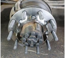
11. Mount wheel onto 8 to 10 Lug adapter using a 33mm socket.
