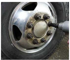
3. Use brake cleaner and wire brush to clean off the factory adapter and wheel studs.
