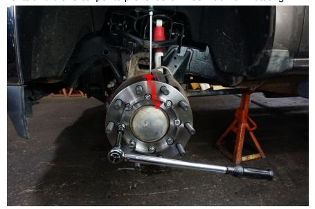
**9.** Mount wheel onto 8 to 10 Lug adapter. Make sure that none of the factory studs are coming into contact with the wheel. Fasten the wheel using a 33mm socket.
