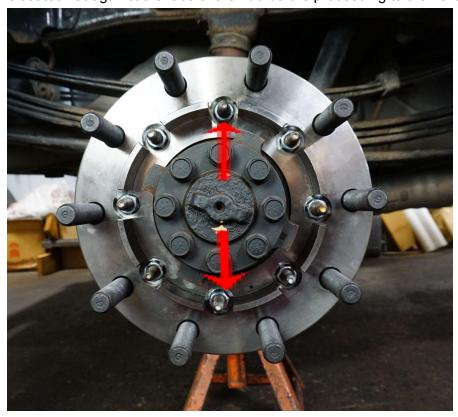
**6.** Next, use a paint marker and a thin straight edge (we used a 0.010" feeler gauge) to mark the cut off location on each of the factory hub studs. Let the paint dry before removing the nuts.
