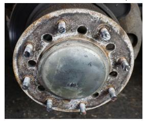
8. Mount the 8 to 10 lug adapter using the provided red loctite. Using a % socket, torque the eight M14x1.5 nuts to 145 ft.lbs. A screwdriver can be placed in the brake rotor vents and brake caliper to prevent the wheel hub from rotating.
