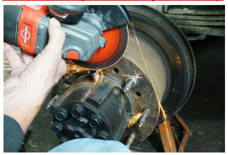
9. Remove the M14x1.5 nut this will help clean up any burrs on the stud left from cutting.
