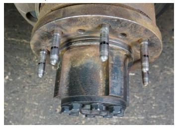
8. Screw a nut onto each of the studs **before** cutting them. Use a metal cut off wheel to cut the studs at the paint marker line. *The studs will be hot! Use caution before touching* them and wait until they cool before moving onto the next step!
