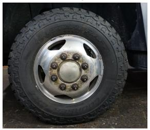
**2.** Raise vehicle using a hydraulic lift or jack <u>and supporting jack stands.</u> Use an impact gun to remove the wheel.
