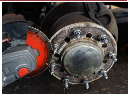
7. Remove the M14x1.5 nut this will help clean up any burrs on the stud left from cutting.
