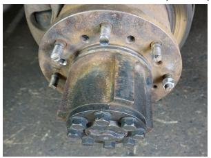
**10.** Mount the 8 to 10 lug adapter using the provided red loctite. Torque the eight M14x1.5 nuts to **145 ft.lbs.**
