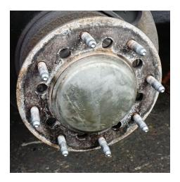
**4.** Thread on a M14x1.5 nut all the way down to the face of the factory adapter, then thread on a second nut down until it meets the first. The height of the two stacked nuts will ensure that sufficient stud length is left after cutting the studs.
